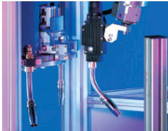
1 Robot docks WH neck into ATS-Rotor change station.
