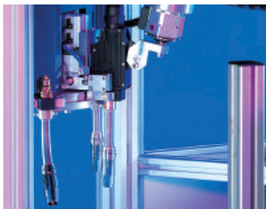
3 The change neck is taken off by the downward movement of the rotor plate. Quick release valves in the water channels avoid leaking of the coolant.
