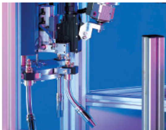
3 The change neck is taken off by the downward movement of the rotor plate. Quick release valves in the water channels avoid leaking of the coolant.
